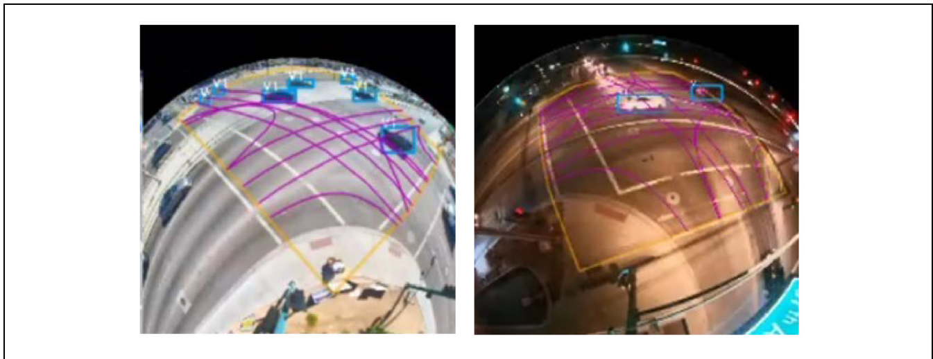
Figure 3. The smart sensors' detection overlay configuration.
